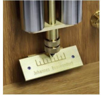
A view of the beautiful pendulum scale that illustrates the pendulum deflection. A uniform oscillation amplitude ensures the accurate running of the clock. The scale shows the oscillation amplitude. Ideally, this should be the same in both directions.
