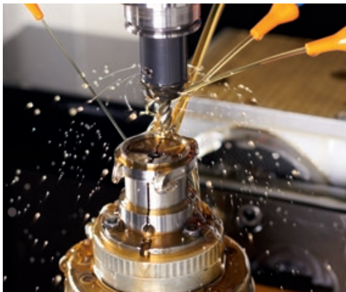
Machining a watch case using a state-of-the-art CNC machine.
