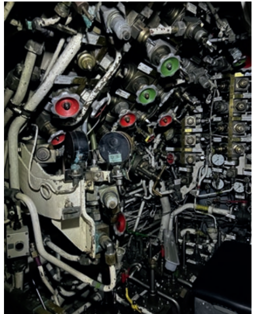
View of the trim system of the Type 206 A U 15 submarine. One of the tasks of the trim system was to adjust and monitor the weight of the underwater vessel.
