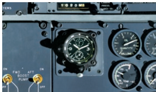
SINN navigation onboard clocks were also used in civil aviation. Shown here is the NaBo 17 ES in the cockpit of a Boeing 727.
