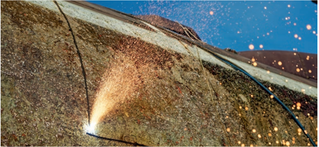
The first step in the recycling process at KSH: A flame cutter is used to cut out steel plates from the U 15's hull.
