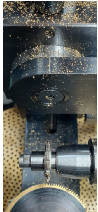
Cutting the wheel teeth on a wheel blank using a milling module.
