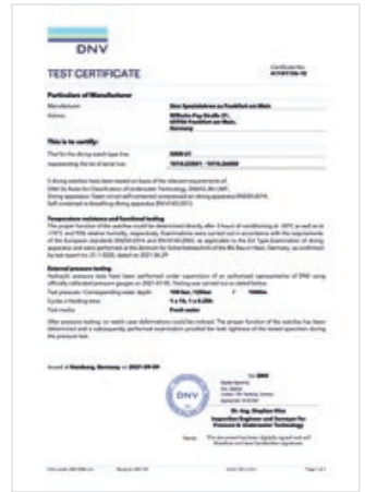
DNV verifies and certifies the pressure resistance of our U1 SL to a diving depth of 1000 m and the temperature resistance and functionality based on European diving equipment standards EN250 and EN14143.
