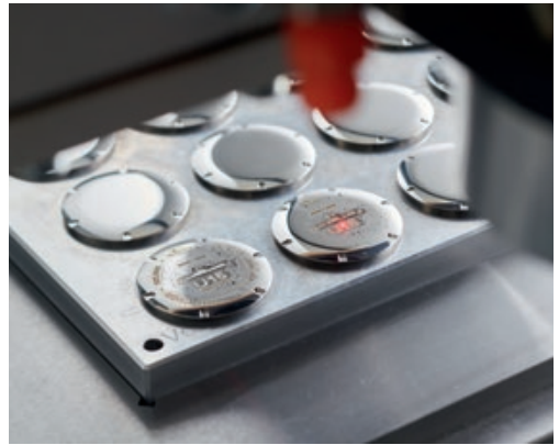
The intricate engraving on the screwed back, made using a precision laser system.
