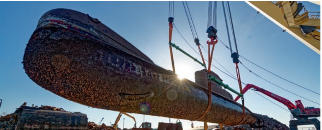
The floating crane lowers the U 15 – which weighs some 450 tonnes – into the so-called cradle. Here, the submarine is kept stable until the hull is dismantled.
