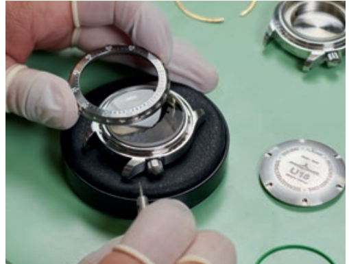
During final assembly, the individual components are pieced together to form complete cases.
