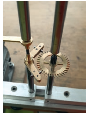
The Graham escapement prevents the wheel train from moving too quickly or in an uncontrolled manner.
