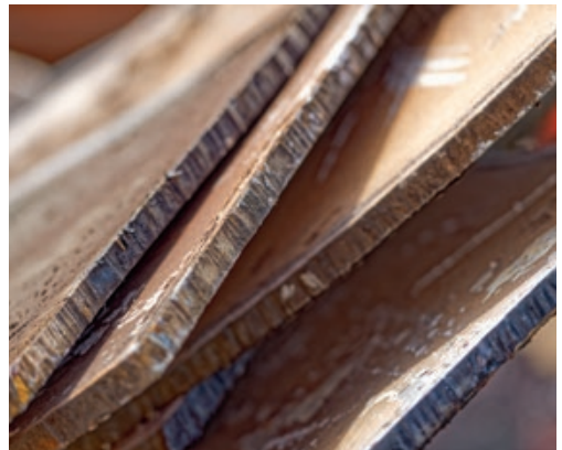
Cut-out plates of non-magnetic German Submarine Steel, which still need to be straightened for further processing.
