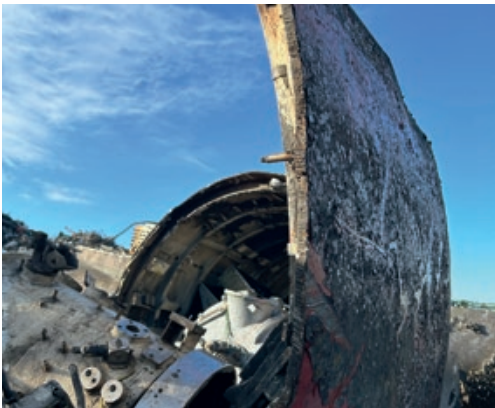
The inner wall thickness of a Type 206 submarine is much thinner than you might think thanks to a sophisticated stiffening structure.
