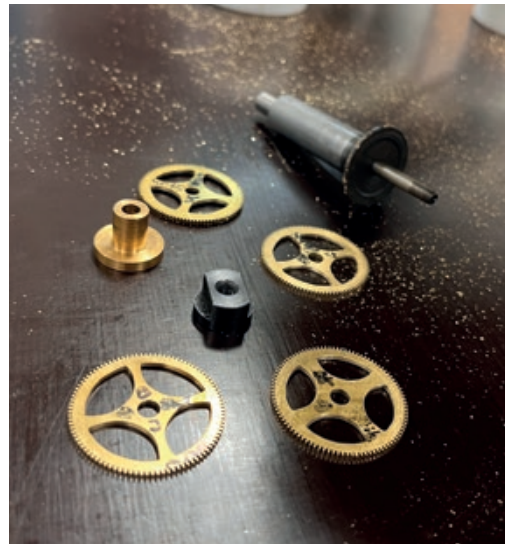
Made by the trainees themselves, these wheels are responsible for force transmission inside the movement.
