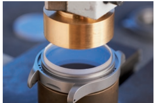
The utmost precision is required when pressing in the sapphire crystal glass.
