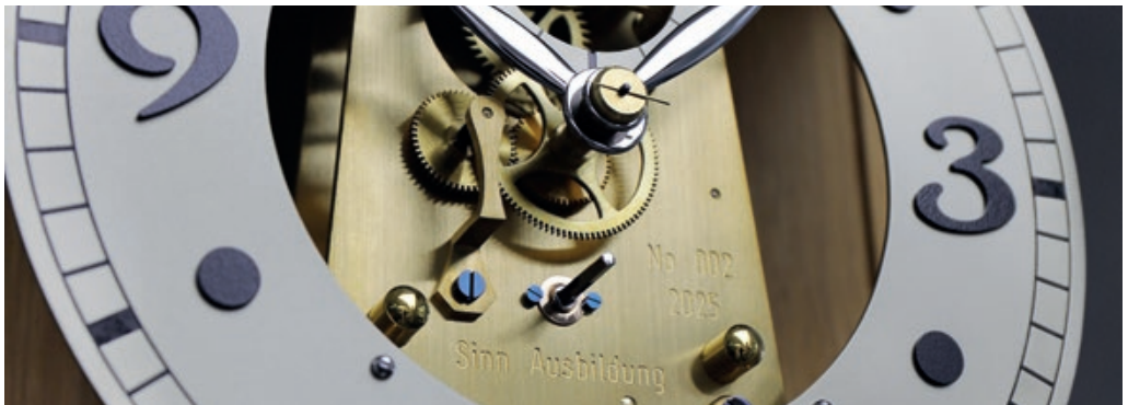
The dial of the pendulum wall clock is made of German silver. The indices are crafted from brass: they were first filed by hand and then finished with a black lacquer. The hands, by contrast, are made of steel and were polished to a high gloss in a subsequent step. The design of the dial was conceived and executed entirely by the apprentice himself.
