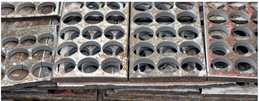
Optimal material utilisation thanks to CAD-controlled water jet cutting system. The leftover pieces are also recycled.
