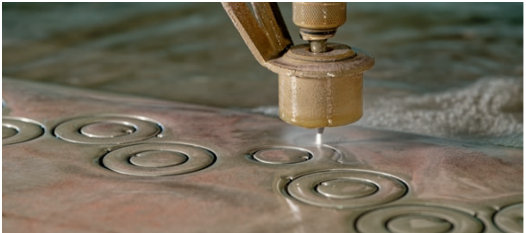
A water jet cutter is used to cut out the blanks for the case back and middle and the rotating bezel from the straightened plates of German Submarine Steel.
