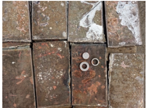
Straightened steel plates from the U 15 submarine and the resulting blanks in various dimensions.
